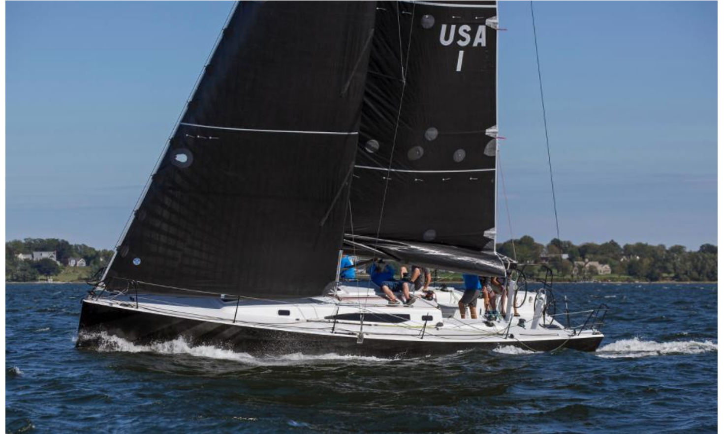
Non Overlapping Jibs (J1, J2, J3, J4 - overlap is similar, but change in shape and weight)
